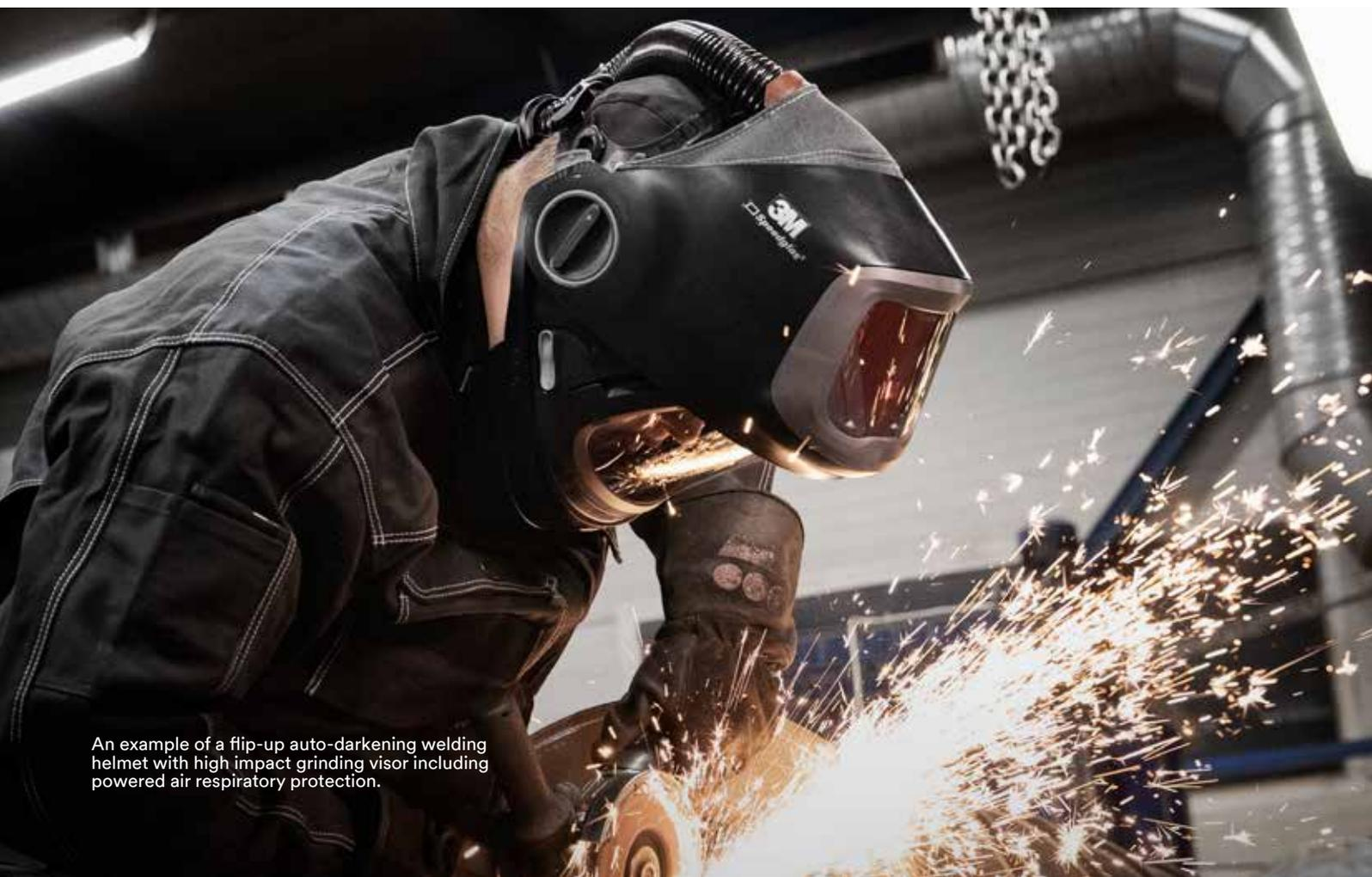
An example of a flip-up auto-darkening welding helmet with high impact grinding visor including powered air respiratory protection.
